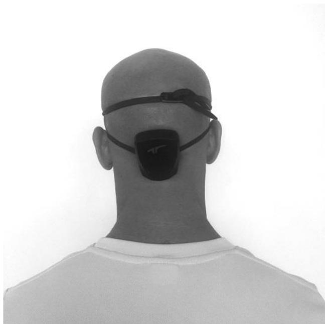
**Fig. 1.** Placement of TritonWear<sup>®</sup> device fitted directly inferior to the inion, on the occipital bone.
